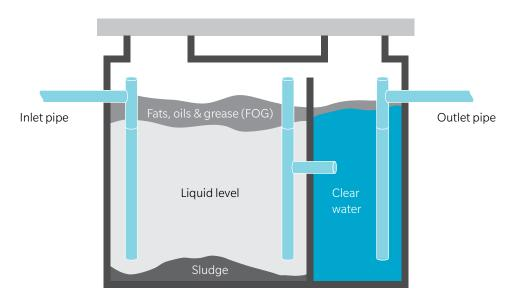
Grease trap: scheme of work
